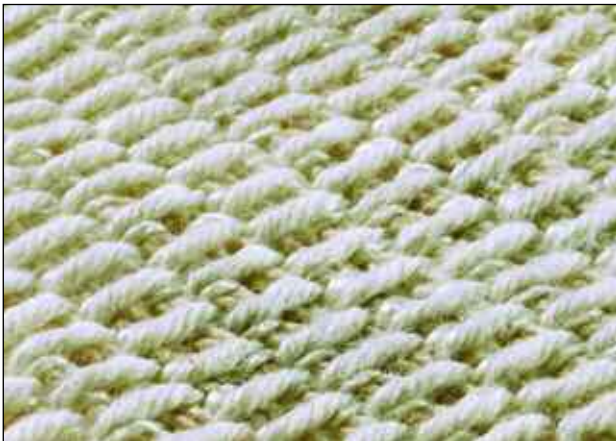
Solid-woven carcass prior to PVC impregnation
